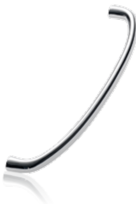
MINIMAL 531760160 Design Jesper K. Thomsen Material Zamac Finish 08 - Bright chrome / 66 - Inox look Centre distance 160 Length 170 Width 8 Height 33
